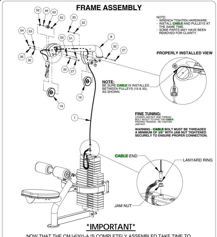
NOW THAT THE CMJ-6201-A IS COMPLETELY ASSEMBLED TAKE TIME TO ASSURE THAT YOUR UNIT IS ASSEMBLED SQUARE AND PERPENDICULAR. USE A LEVEL TO CHECK THAT THE GUIDE RODS ARE PERPENDICULAR IN BOTH DIRECTIONS. IF THEY ARE NOT PERPENDICULAR IN BOTH DIRECTIONS, IT WILL BE NECESSARY TO LOOSEN SOME FRAME HARDWARE TO RE-ALIGN THE FRAME AND RETIGHTEN BOLTS.
