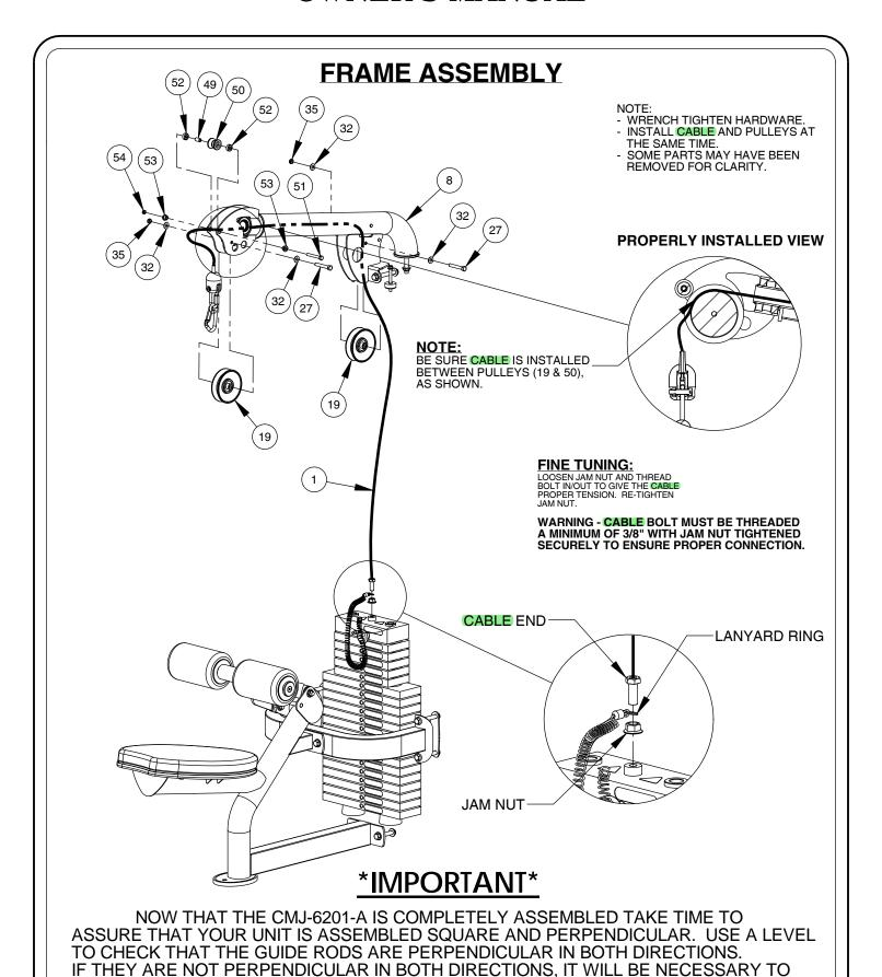
LOOSEN SOME FRAME HARDWARE TO RE-ALIGN THE FRAME AND RETIGHTEN BOLTS.
